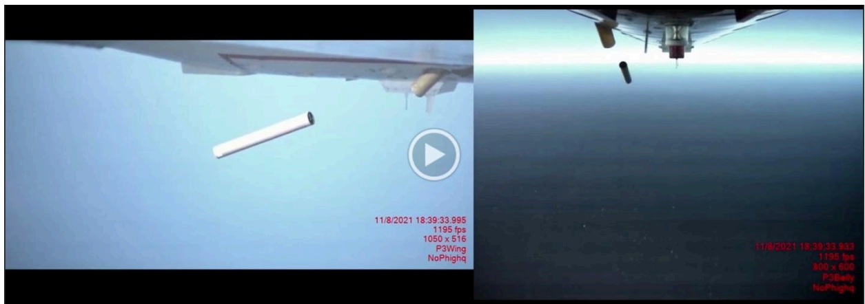
Picture showing the deployment of ADWSD™ from NOAA’s AOC P3
