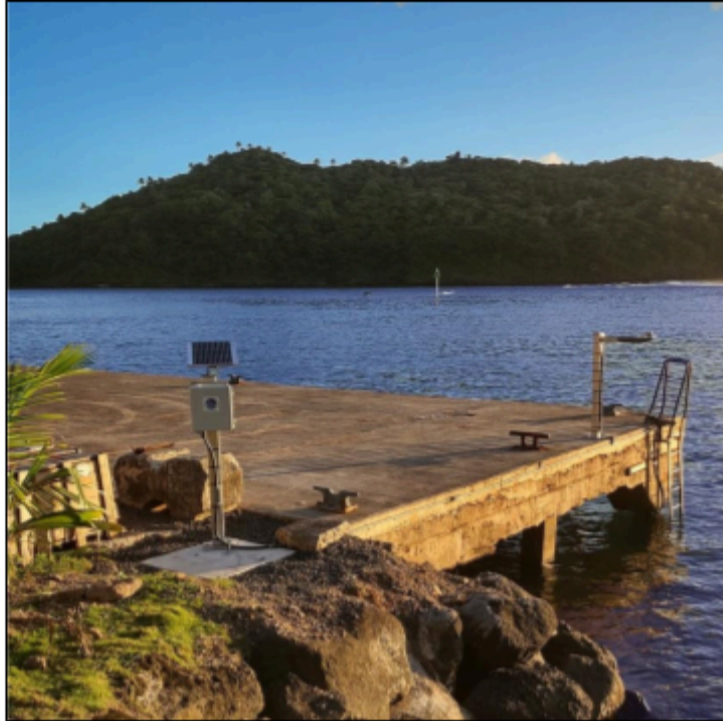
Figure SEQ Figure \* ARABIC 2: Photo of the new UHSLC tide gauge installed on the island of Ofu in the remote Manu'a Islands, which are part of American Sāmoa.
